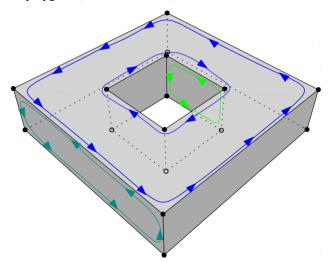
In other words, the normal of the surface must point outwards if a right-hand system is used, ie when the ordering of points follows the direction of rotation of the curled fingers of the right hand, then the thumb points towards the outside. If the polygon has interior rings, then these have to be ordered clockwise.
