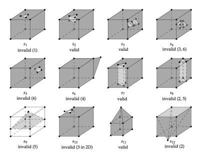
The first assertion means that a solid must be closed, or 'watertight' (even if it contains interior shells). The solid  $s_1$  is thus not valid but  $s_2$  is since the hole in the top surface is 'filled' with other surfaces.
